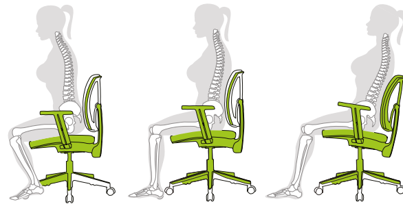
The centre of gravity in different seating positions
